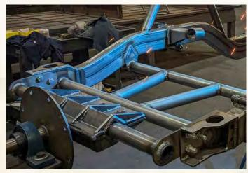
Heavy Duty Polyurethane Bushings Heavy wall polyurethane bushings limit engine movement and reduce vibrations.
