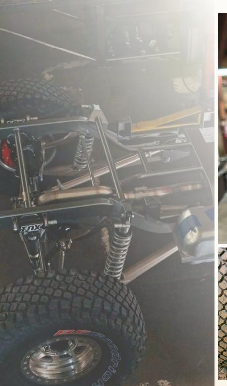
To match the capabilities of the front suspension, while providing a better feel for the road and a comfortable ride our triangulated rear offers tremendous adjustability to help control a vehicle's handling on various surfaces and conditions. Utilizing "triangulated" upper bars, our rear suspension is engineered to keep the rear end centered under your rig to maintain stability and control even under hard acceleration, rock crawling and cornering.
