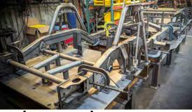
chassis is produced precisely and accurately. Every chassis is created in robust tooling weighing several thousand pounds.
