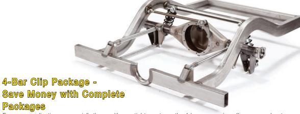
For many applications - especially those with very tight quarters - the 4-bar suspension offers many advantages. Operating on the principle of a constant motion parallelogram, the design of the 4-bar is such that the rear end housing is always parallel to the ground - pinion angle never changes.
