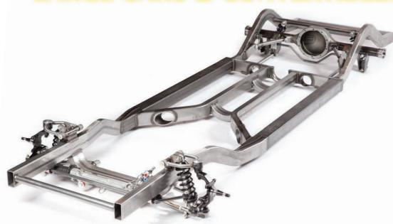
Size does matter and Art Morrison Enterprises offers heavyduty chassis for long wheelbase cars and convertibles with 4"x4"x.180" wall main rails. This provides the extra rigidity needed to improve the handling and ride quality of larger
