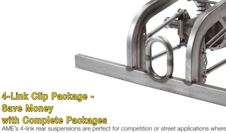
AME's 4-link rear suspensions are perfect for competition or street applications where maximum adjustability is desired. There are six upper bar front mounts plus four lower bar attachment holes, along with two top and bottom housing mounts and adjustable bars to provide you with any instant center point desired.
