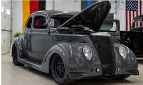
This 1937 Ford Business Coupe built by Anton's Hot Rod Shop carries more custom pieces than we can list. Equipped with a full AME chassis, it is powered by a 6.2L LS3 backed by a 6L80. antons\_hotrod\_shop Photo By: Maddie Dobay. sofinemadoline
