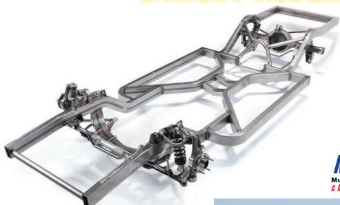
Art Morrison Enterprises developed the MaxG chassis as an effective means of providing sports car-like handling and a contemporary, aggressive stance to owners of classic unibody-chassied muscle cars. A large number of cars manufactured by AMC, Chrysler, Ford and General Motors in the 1960s, '70s and '80s featured unibody construction. We have engineered MaxG chassis for the majority of them.
