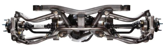
There are inherent benefits that come with an independent rear suspension, such as improved handling and ride characteristics. However, not all IRS designs are equal. Early IRS setups, typified by Jaguar, Cobra and C2/C3 designs have shortcomings when it comes to toe and camber control, limited spindle and anti-squat support, wheel offsets and overall space considerations.
