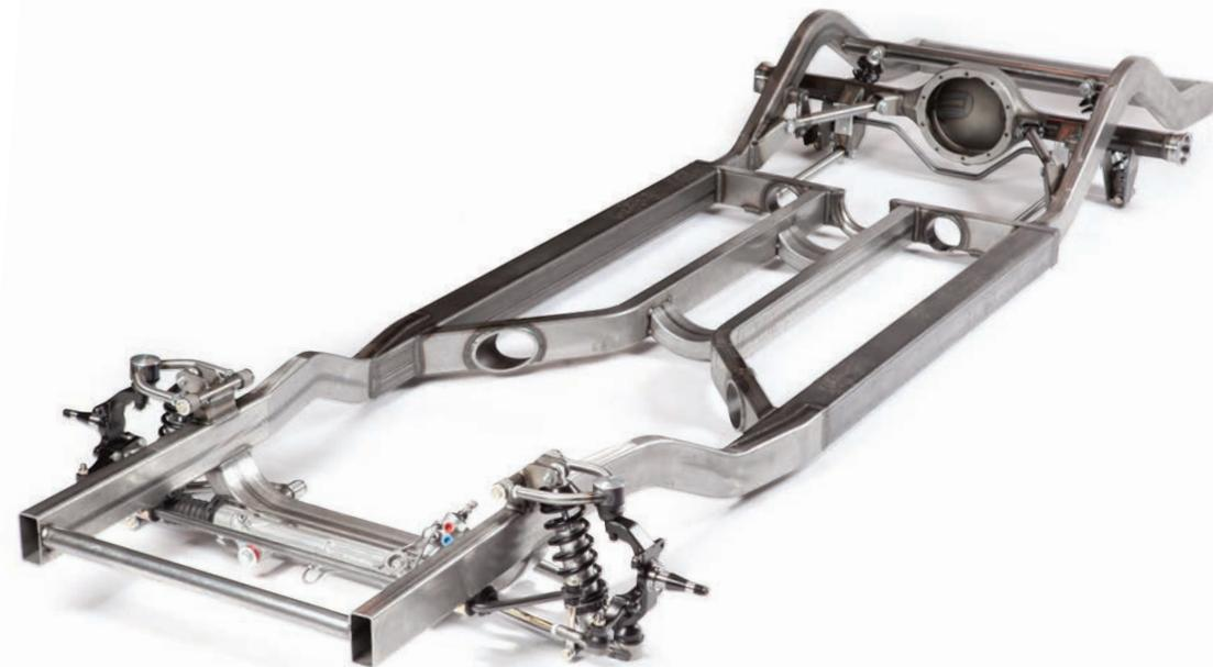
Size does matter and Art Morrison Enterprises offers heavy-duty chassis for long wheelbase cars and convertibles with 4"x4"x.180" wall main rails. This provides the extra rigidity needed to improve the handling and ride quality of larger vehicles.
