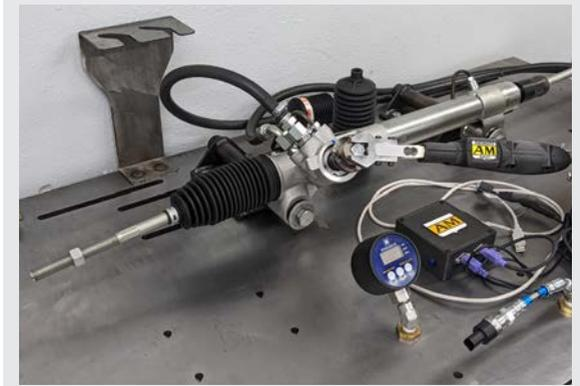
AME has a special steering dyno to test and evaluate components.
