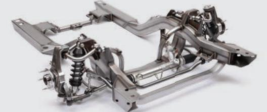
angles for use with aggressive, low treadwear-rated tires. This new setup also features serviceable ball joints and employs high strength steel coilover mounts to withstand high stress cornering and bump loads.
